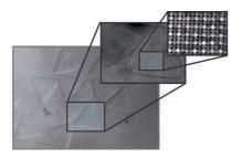
Assembly-line microparticles: An innovative approach for the high-throughput fabrication of complex three-dimensional and chemically anisotropic microstructures is highlighted (illustrated: patterned triangles with edges of circa 60  $\mu$ m) based on the synergistic use of stop-flow interference lithography and microfluidics.
